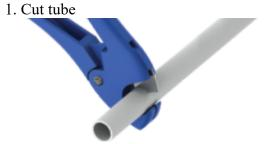
Cut the tube square and remove burrs and sharp edges. Ensure the outside diameter is free of score marks. For soft or thin
