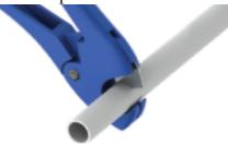
Cut the tube square and remove burrs and sharp edges. Ensure the outside diameter is free of score marks. For soft or thin walled tube we recommend the use of a tube insert. 2. Push up to tube stop
